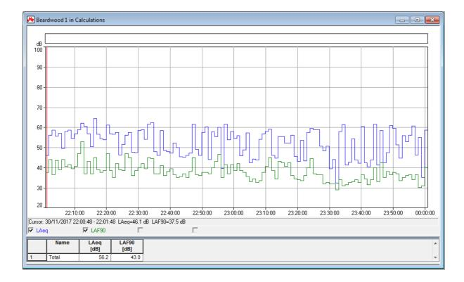
As can be seen the measured LA eq between 22.00 and 00.00 was 56.2 dBA ( T = 1 minute ) - the peaks on the graph representing the passage of car / cars passed the measurement location.
