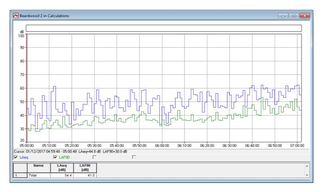
As can be seen the measured LA eq between 05.00 and 07.00 was 54.4 dBA (T = 1 minute) - the peaks on the graph representing the passage of car / cars passed the measurement location.
